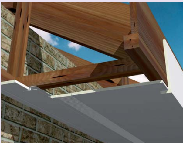
9mm Square Edge Fascia – Vented multi-purpose board as a soffit
